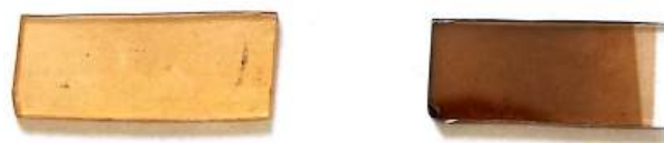
Figure 1: Surfaces of the undoped (left) and Cu-doped (right) Fe 2 O 3 deposited films taken by an optical camera Camon 12 Pro.
